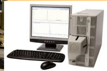
FIG. 1. Photograph of the Microscopic Systems 3500 MID miniature mass spectrometer, showing the small footprint of the instrument. Photo courtesy of Microscopic Systems PLC.
